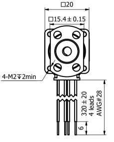
Step angle 1.8° Rated current/phase 0.5 A 5.1Ω±10% Resistance/phase Inductance/phase 1.5 mH±20% 0.01mm/step Linear travel per step Ball screw diameter Ф4.0mm Ball screw lead 2.0mm C7(KSS) Grade Insulation class 100MΩ(500VDC) Insulation resistance Heat rise 80°C 0.08 kg Motor weight
